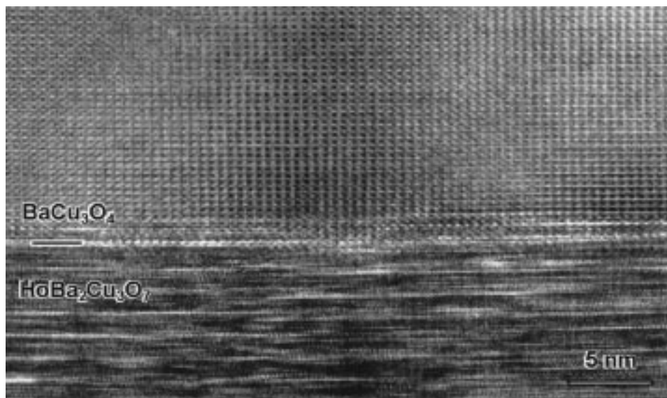
Figure 9. HREM image of the BaCu 3 O 4 /HoBa 2 Cu 3 O 7-δ interface along [110] HoBCO , whereas BaCu 3 O 4 is in [010] orientation. The interface is sharp and shows no additional phases. c axes of BaCu 3 O 4 and HoBa 2 Cu 3 O 7-δ are parallel.
